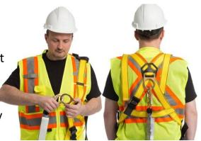
Follow the manufacturer's instructions on how to care for and clean the components of the fall arrest system, including the body harness.
